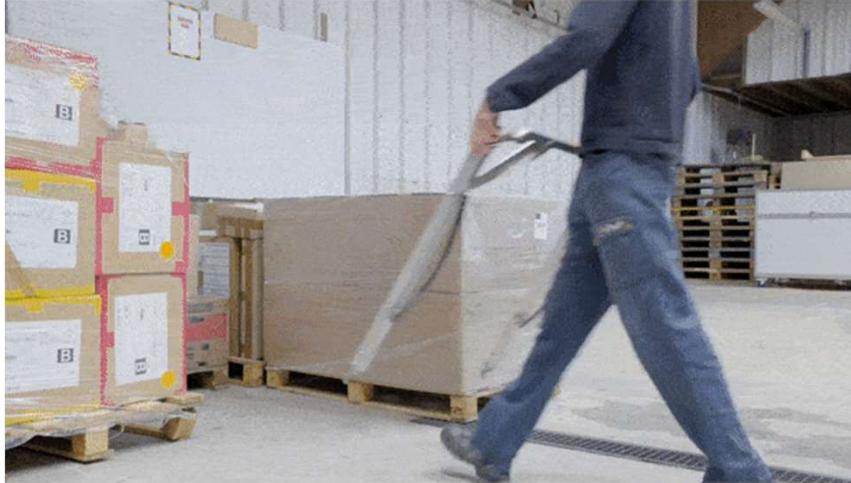
BicyLift (FlexiModal): an innovative bike trailer designed for cycle logistics and compatible with the EUR-pallet standard Watch the full video on https://youtu.be/F9dw9gQJuxU
